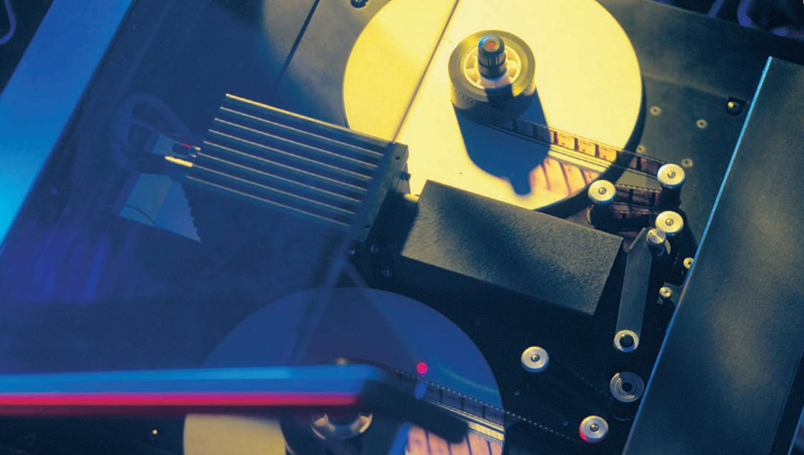
The GOLDEN EYE film scanner is a high resolution digitizing unit for 16 and 35 mm Cine or Picture film.
